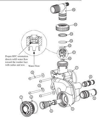
WS1.5 and 2L Refill Flow Control Assembly and Refill Port Plug
