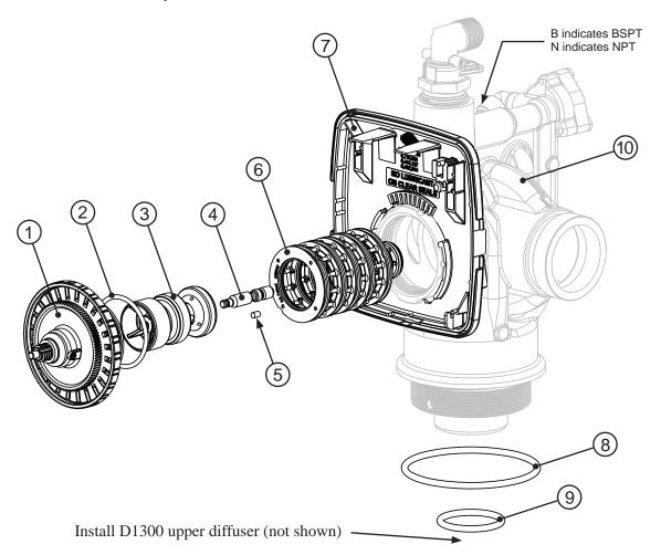
WS2 Drive Cap Assembly, Downflow Piston, Regenerant Piston, Spacer Stack Assembly and Main Body
