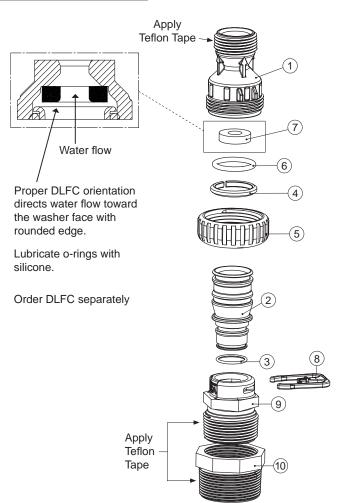
V3053 WS2 2-1/2 GROOVELOCK CLAMP ASY
