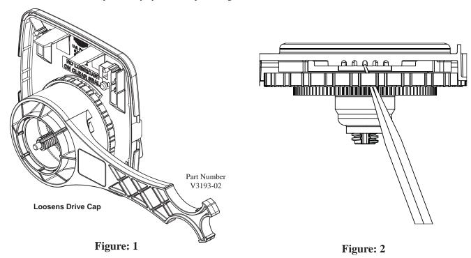
The drive cap assembly contains the drive cap, the main drive gear, drive cap spline, piston rod and various other parts that should not be dissembled in the field. The only replaceable part on the drive cap assembly is the o-ring. Attached to the drive cap assembly is the main piston (down flow) and if a regenerant is used, a regenerant piston.
