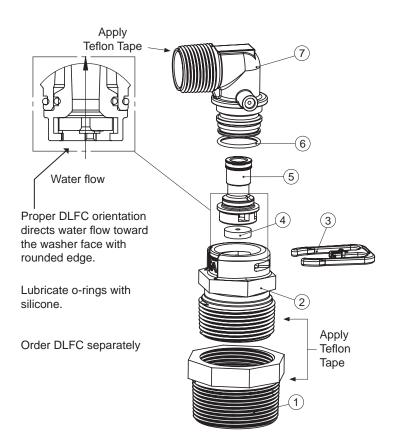
V3008-05 WS2 Fitting Drain 1" Male NPT Straight Without Silencer
